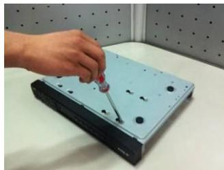
5. Fix the HDD firmly.
