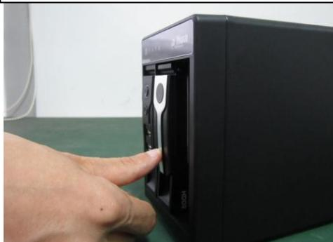
④ Put the knob back after you insert the HDD to the SATA board.
