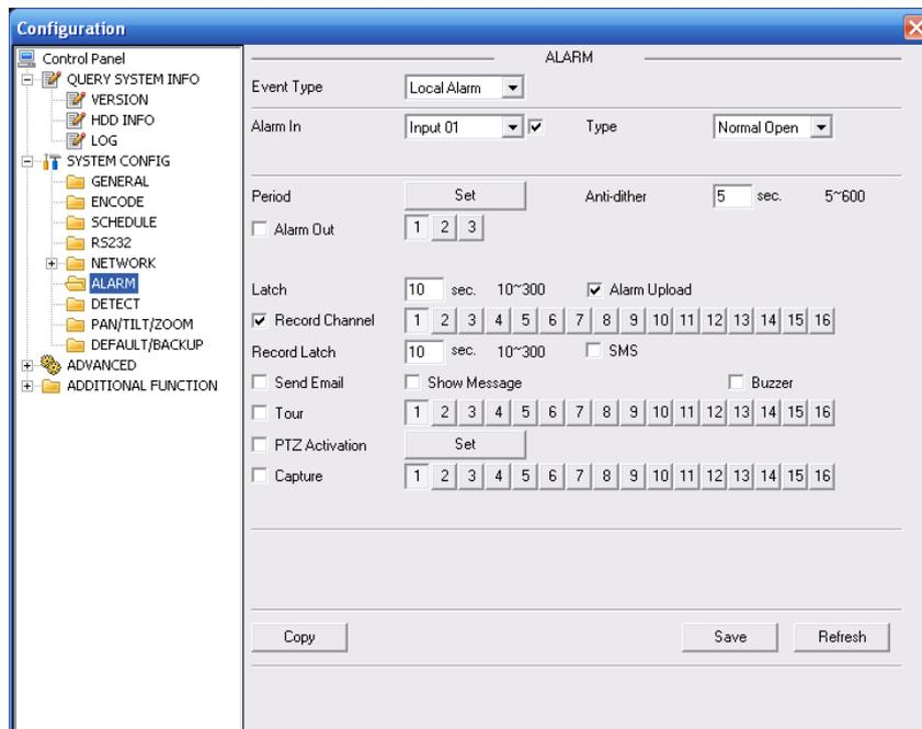
Figure 8-39 Alarm Setup
