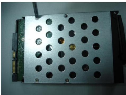
① Use 4 screws to secure the HDD
