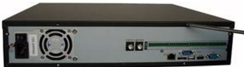
① Use the screwdriver to loose the screws of the rear panel and then remove the front cover.
