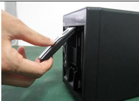
③ Pull the HDD knob up when you put the HDD into the box in case the knob buckle may strike the front panel.
