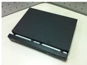
7. Put the cover in accordance with the clip and then place the upper cover back.
