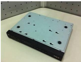
4. Turn the device upside down and then turn the screws in firmly.
