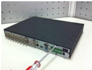
1. Loosen the screws of the upper cover and side panel.
