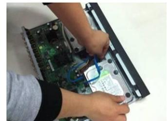
6. Connect the HDD cable and power cable.
